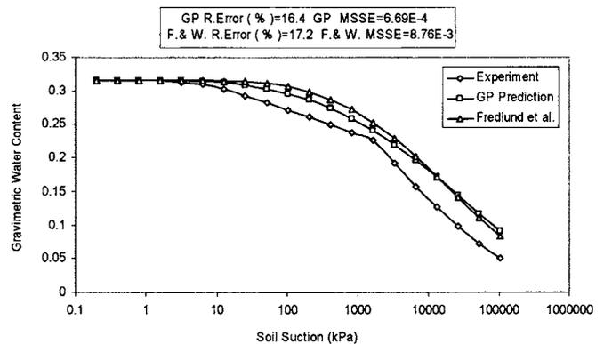
**Fig. 6.** Average simulation results among tests used for validation (void ratio: 0.852; initial water content: 31.57%; clay content: 70.33%; silt content: 23.7%; dry density: 1,457.7 kg/m<sup>3</sup>; specific gravity,  $G_s$ : 2.7)
