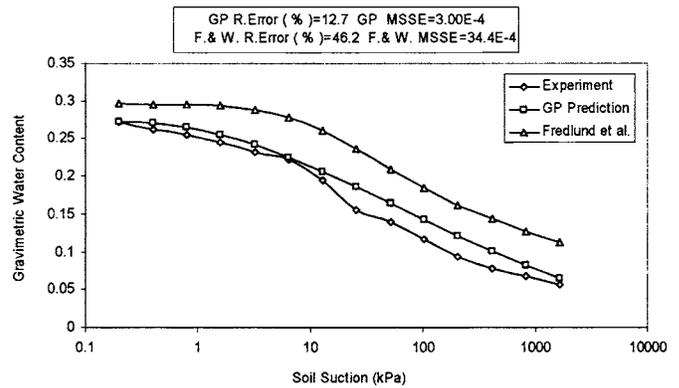
**Fig. 5.** Average simulation results among tests used for developing GP model (void ratio: 0.8; initial water content: 27.23%; clay content: 16.98%; silt content: 75.23%; dry density: 1,500 kg/m<sup>3</sup>; specific gravity: 2.7)
