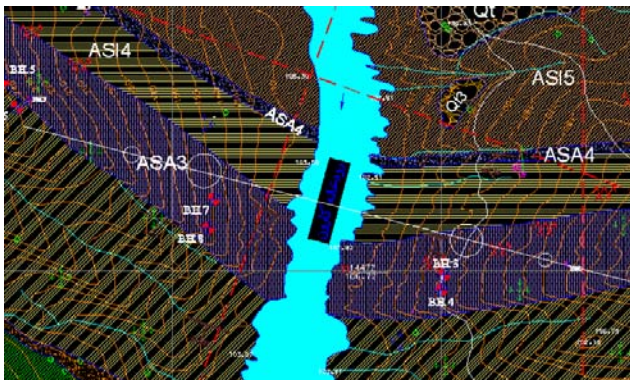
Figure 1. Rock Mass unit ASA3 foundation of rock socket for bridge
