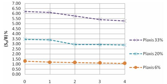
Fig. 7 Variation of  $(S_d/B)$  with number of reinforcement layers with geogrid
