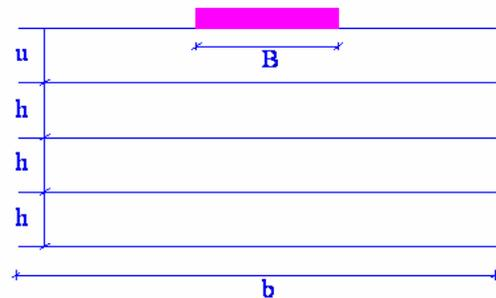
Fig. 1 Shallow square foundation supported by geogrid-reinforced sand
