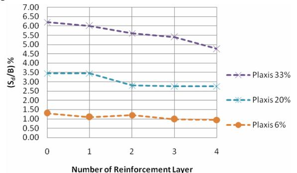
Fig. 8 Variation of  $(S_d/B)$  with number of reinforcement layers with grid-anchor
