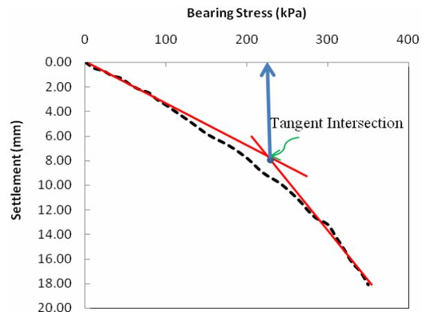
Fig. 3 Load settlement curve for unreinforced soil
